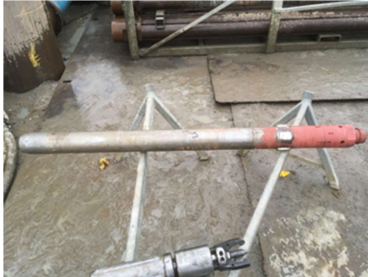
Figure 28. Picture of the coring device that was used to obtain the core samples.
