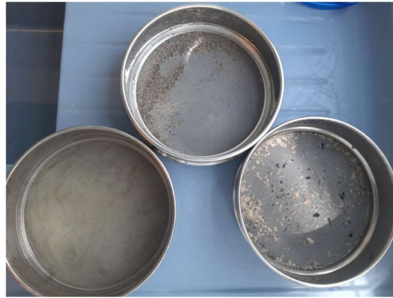
Figure 6. Sieves used to filter real water from industrial complex discharge network.
