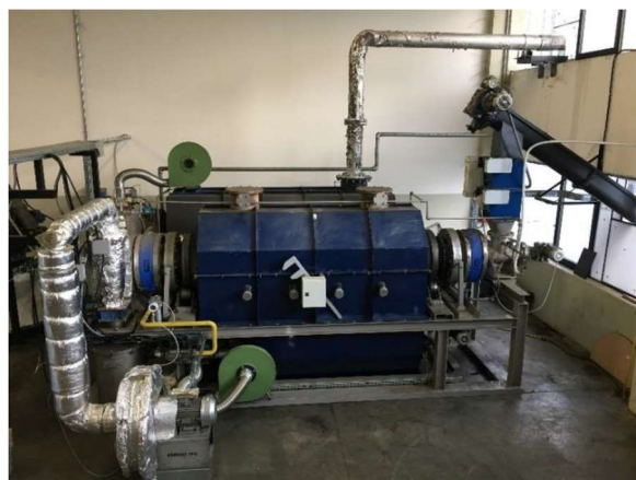
Figure 38. Rotary kiln for slow pyrolysis (PYROCK).
