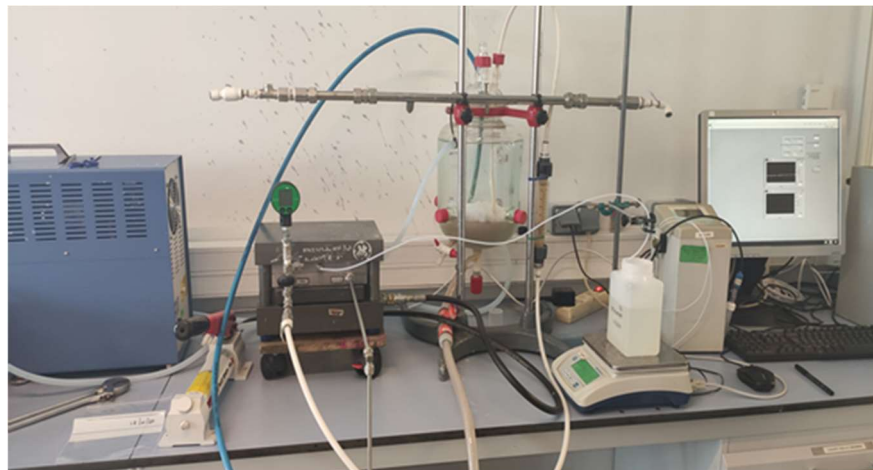
Figure 11. Reverse Osmosis laboratory experimental set-up.
