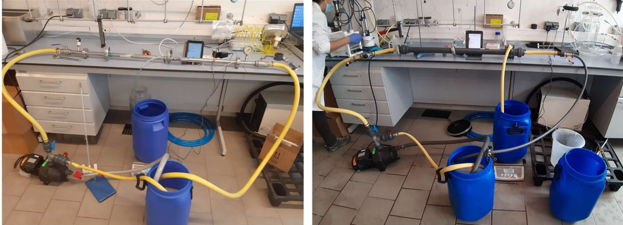
Figure 7. Ultrafiltration experimental set-up. Left: ceramic membrane (1000 kDa), right: polymeric membrane (150 kDa).
