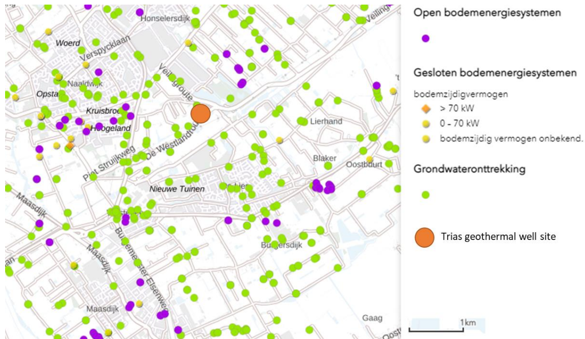
Figure 19. Existing ATES and BHE systems ( www.WKOtool.nl )
