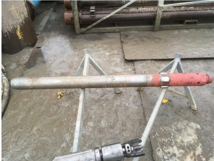
Figure 22 Picture of the coring device that was used to obtain the core samples. The left part is the cutting shoe that goes down into the borehole. The right (red) part is hammered with a weight to push it in the ground. When full, the red top is grabbed using the grabbing device (bottom) and subsequently hinged to the surface. To prevent the sediment from falling out, a check-valve is installed in the bottom of the coring device.
