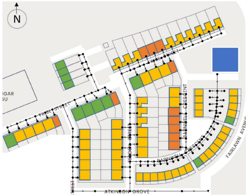
Figure 78 Sewer network overlaid onto housing map (SWMM)
