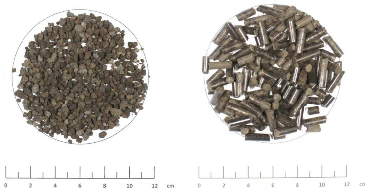
Figure 30 Left: feedstock before pelletising; right: pelletised sludge
