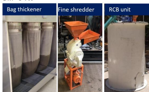
Figure 92 NextGen technologies for material recovery from sludge with dry matter (DM) contents of their inflow streams
