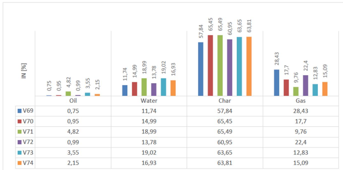
Figure 31 Mass balance (values given in mass-%)
