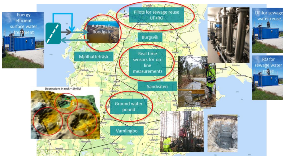
Figure 131: Besides the infrastructure for real-time measurement of the water balance, the following four parts will be included in the pilot system: 1/ Automatic floodgate for storage of water from winter to summer 2/ Treatment of surface water for drinking water supply. 3/ Sewage water reuse in Burgsvik by UF+RO 4/ Groundwater pond for secure, local water supply
