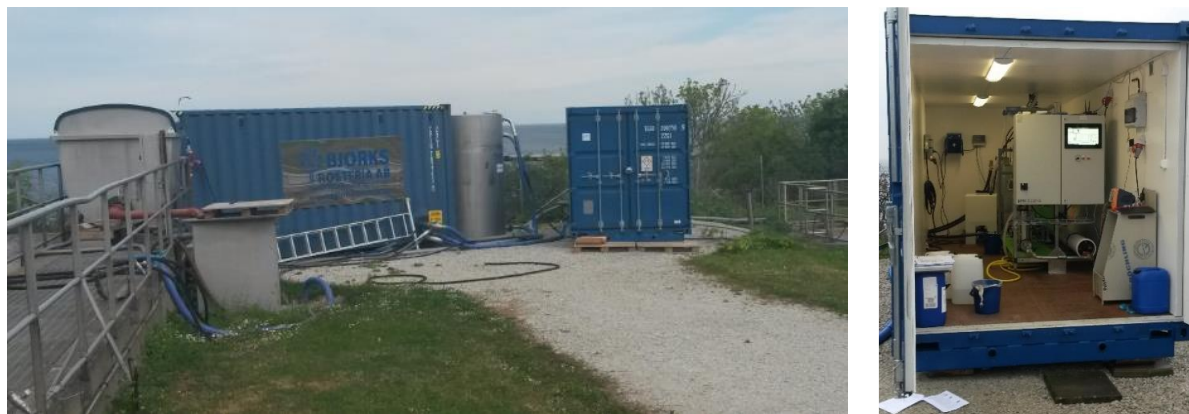
Figure 53. The pilot plant in Visby. On the left image and from left: drum-filter, ultrafiltration unit, buffer tank after UF. The right image depicts the reverse osmosis unit.
