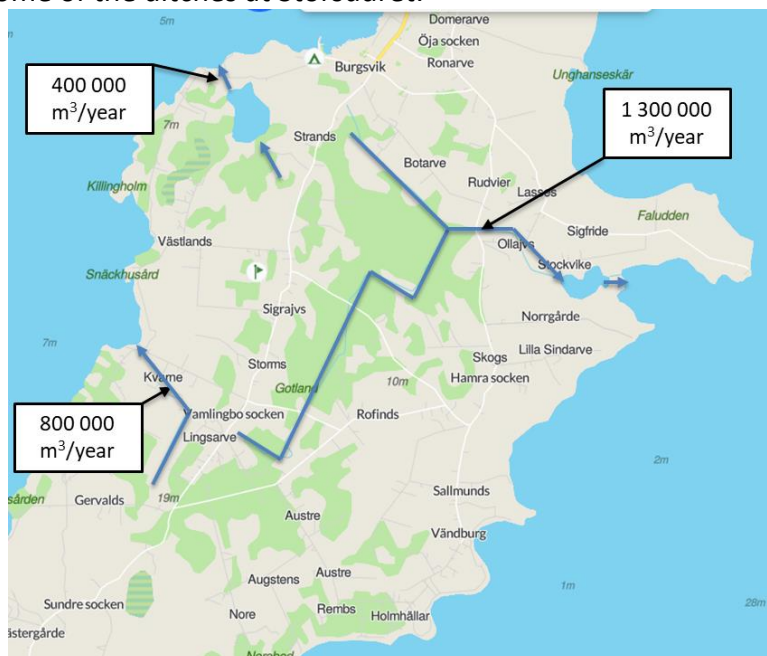
Figure 121. Based on the real time measurements of the flow in the main ditches, the potential of for rainwater harvesting is calculated.
