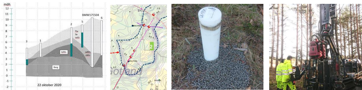
Figure 117. The soil layer profile was established by drilling of several boreholes in area of particular interest for water balance research. In addition, a larger bore hole for making capacity tests was drilled.
