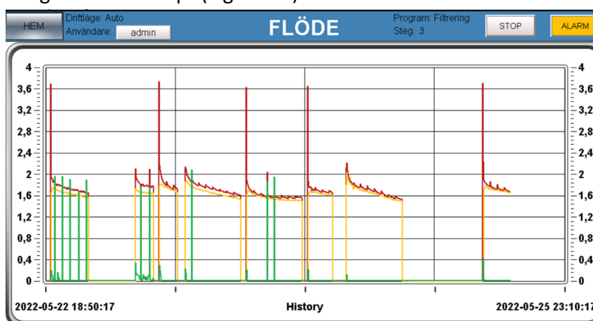
Figure 58. The flow rate ( m^3/h ) of the ultrafiltration unit before and after CEBs.
