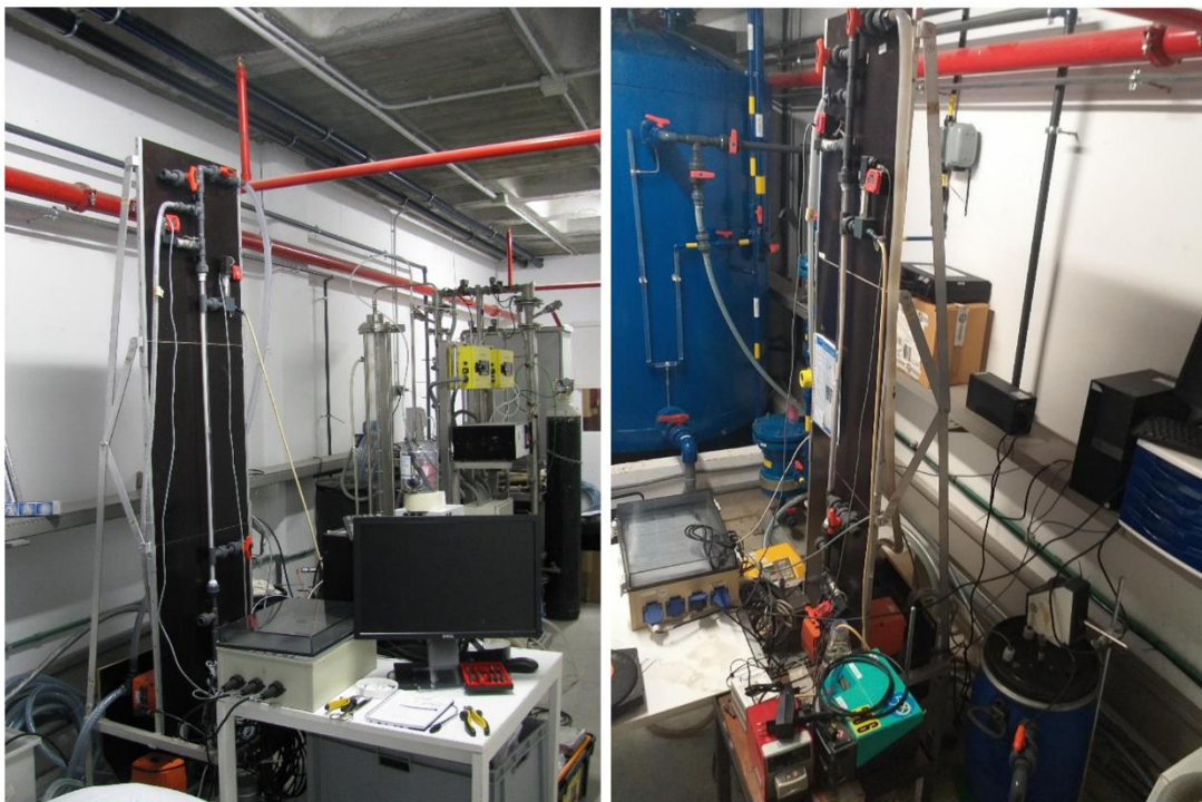
Fig. 2 Pictures of the AnDFCm apparatus (Aqualia)
